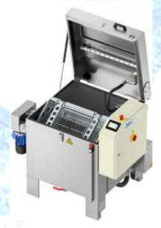
The new Teknox Twister is an ideal washing system for spray washing multiple small components contained in a preloaded detachable stainless-steel basket.
