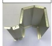
Aircraft part – Machined and fabricated from Titanium material
