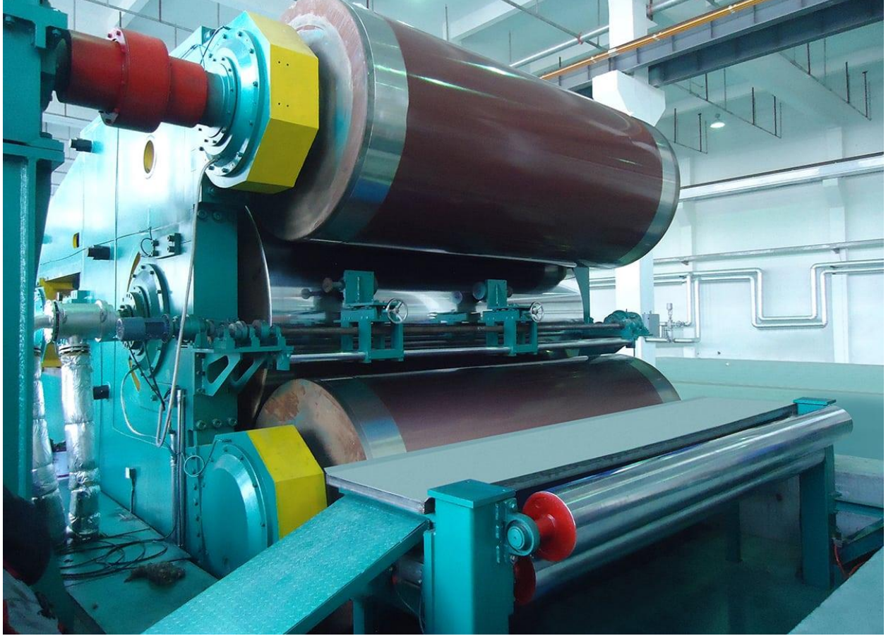
The equipment shown above is a Calender, used in the production of elastomers formed into sheeting.
