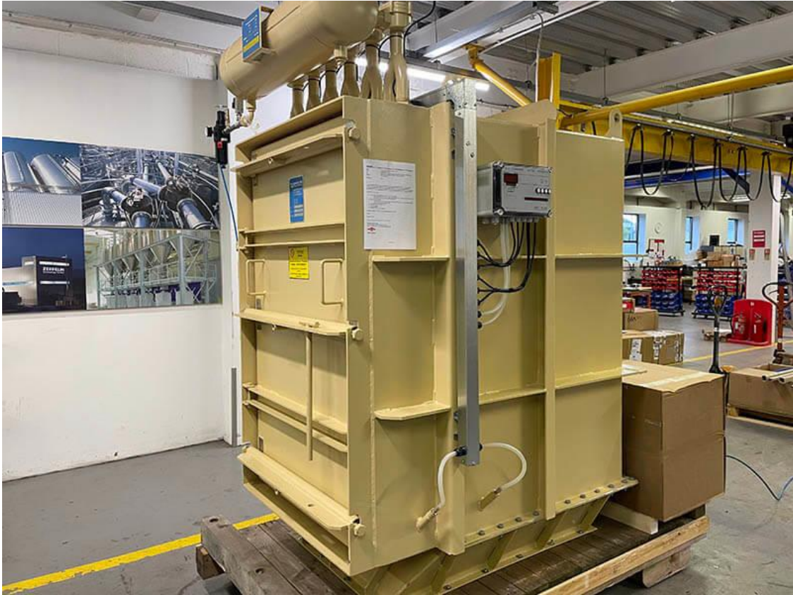
Chemical Plant Silo Venting Filter - South Wales
