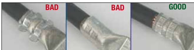
Picture 1: A comparison of good and bad crimps: An incorrect crimp (left: Over compressed, middle: under compressed (leading to increase in resistance), right: correct well formed crimp with die reference visible
