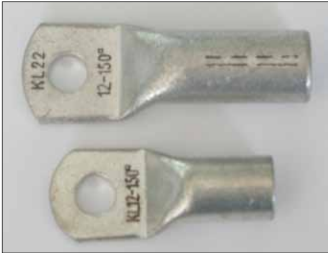
Picture 3: Only DIN compression cable lugs show the required number of crimps stipulated by the manufacturer
