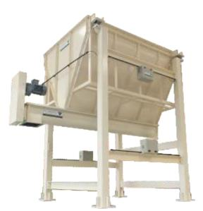
All three weighers incorporate a 4 point loadcell weigh frame with rectangular hopper and a full length discharge screw feeder each with a 2000Kg capacity. Material is discharged from the weighers via flexible connections into linear vibratory screens.
