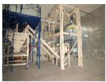
The two external bulk silos each feed directly into two dedicated batch weighers located just inside the building. This is done via screw feeders with automatic shut-off valves passing through the building wall.
