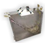
guide and over the top of a single speed drive assembly which draws the stream out of the feed hopper. The assembly comprises of a pair of side wheels with rubberised drive rods between to grip and feed the sachets.
