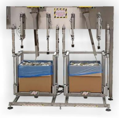
The boxes are located upon a moving carriage system, as the chute swings across the box width the carriage moves backwards and forwards at a constant rate to provide an evenly distributed layer of sachets within the box.
