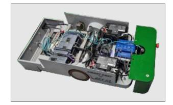
Each AGV is fitted with a high accuracy Mettler Toledo digital scale and an integrated bag clamp assembly. Bags are manufactured by CJ Waterhouse's in-line bag manufacture machine before being swung into position upon the Smart Cart clamp assembly. The clamp assembly is then opened and the carriage sets off, passing under an array of material dosing stations to collect individual ingredients in accordance with the specific recipe.
