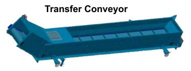
The transfer conveyor resides below the shear roller system and comprises of a fully enclosed flighted belt conveyor which moves the chopped material to the downstream elevating conveyor.
