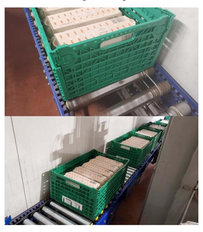
In the fast-paced world of egg production, efficiency and productivity are key factors that can make a significant difference in the success of a business. In a recent Conveyor System manufactured by Mobility Engineering we utilised zero pressure accumulation, a method that offers numerous advantages for egg production lines.
