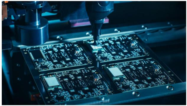
Printed Circuit Board on a Factory Assembly Line with Automated Robotic Arm for Surface Mounting Microprocessors to the Motherboard.
