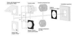
As the above image describes, the Berker sockets and Berker switches are fixed into an application using screws which are then covered from view by the snap fit frame. IP44 protection is available for some sockets when using the hinged cover and seal. Please refer to the Berker catalogue to identify which of the parts are suitable for IP44 – <u>https://www.abcomponents.co.uk/wp-</u>
