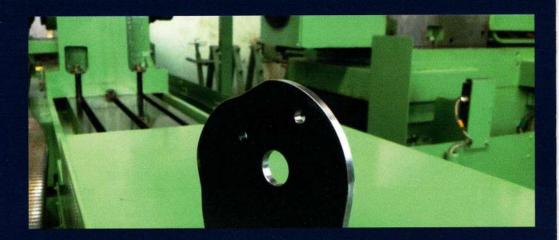
Polgain Limited manufactures cams from a wide variety of materials to suit most heat treatment requirements, working from customer's drawings or supplied samples.
