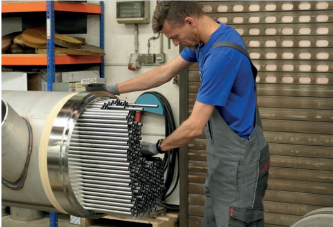
01 In tube heat exchangers, up to 700 tubes are manually inserted and soldered into the tube plate
