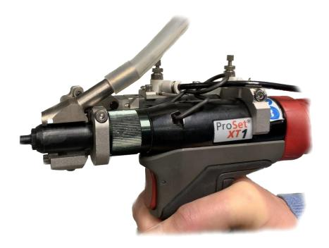
The Z-AR system can accommodate most standard rivet types between 3.0 and 5.0mm diameter, and all rivet materials can be accommodated including aluminium, copper, steel and A2 and A4 stainless steel.
