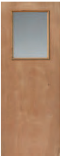
PLYWOOD FLUSH INT/EXT FD30 (KIGOG / KEGOG) 457 x 610mm glazed opening. Pyroshield (Georgian wired)
